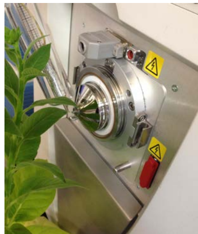
Figure 1. LTP device for the detection of compounds directly from a tobacco plant.
