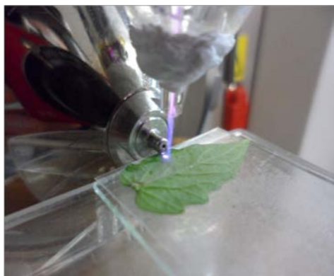
Direct analysis of a tomato leaf with LTP mass spectrometry imaging.
